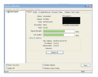
The Link Quality and Signal Strength bar chart is only active when the node is in Infrastructure Mode. The bar graph displays the quality and strength of the link between the node and its Access Point. Link Quality is a measurement of receiving and transmitting performances over the radio. Tx/Rx Frame displays the instantaneous wireless transmitting and receiving throughput in bytes per second.
