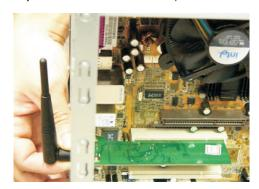
Note: Please make sure that antenna is tightly screwed to get optimal receiving coverage area.
